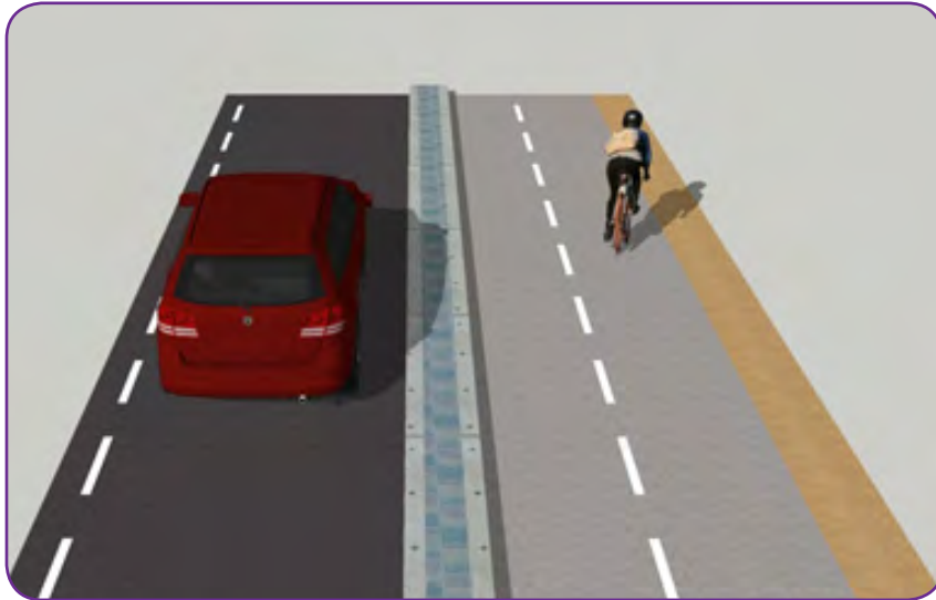
Figure 3-9 Class IV Cycle Tracks
