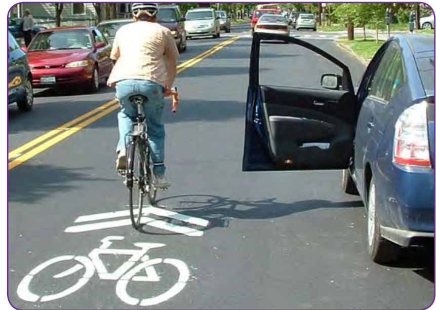
Figure 3-7 Lanes with Sharrow Marking
