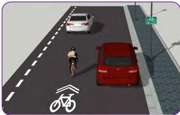
Figure 3-6 Class III Bicycle Facility
