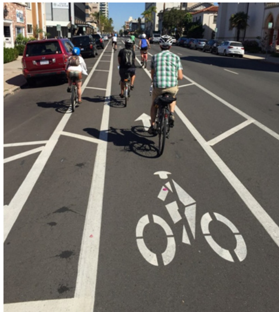
Parking Side and Travel Side Buffered Bike Lane on Fifth Ave, San Diego (Photo: Paul Jamason)
