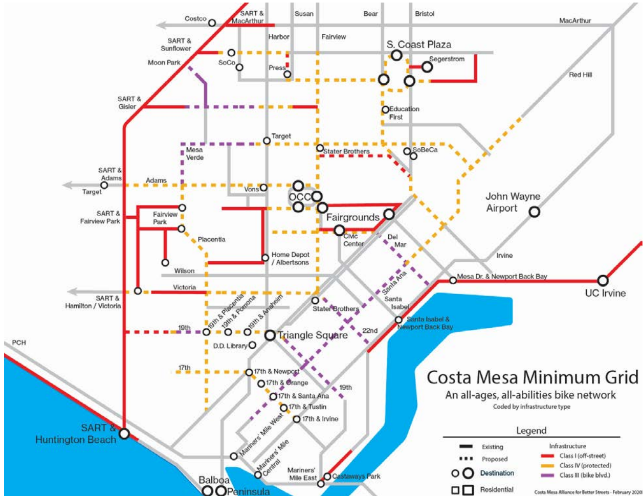
Figure B - Alternative segments for Class III (Boulevard) and Class IV installation, along with existing and proposed Class I facilities, as developed at the February 2020 CMABS meeting.
