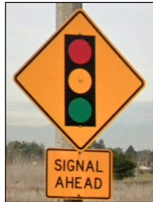
b) Advance warning sign 2 (W3-3 + plaque)
